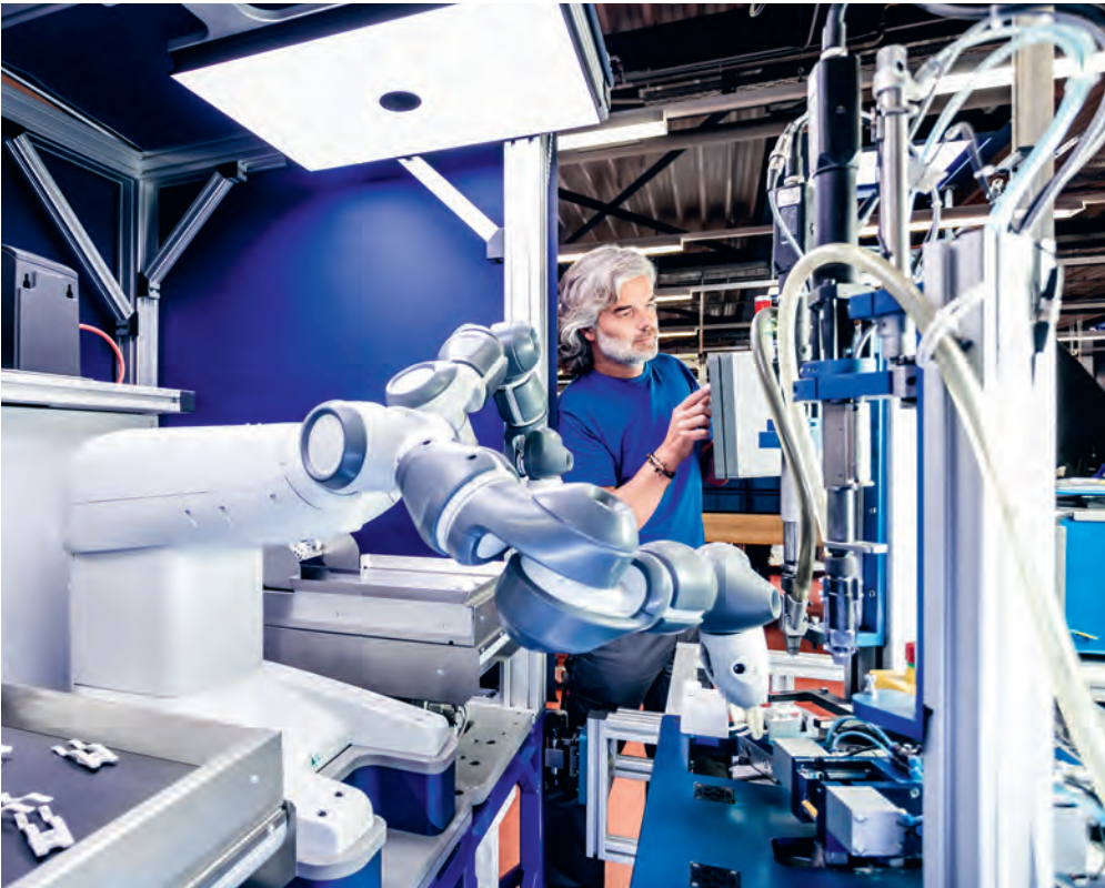
The YuMi robot uses a camera to detect where the parts are and where it has to grip.
