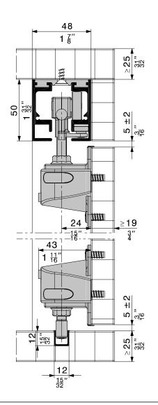
Hardware system for cabinet sliding doors up to 40 kg (88 lbs.). Stacking parallel to the sliding axis.
