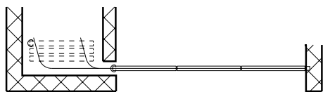
Straight installation with parallel stacking and locking door
