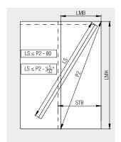
LMB = inside clearance LMH = inside height STB = sliding door width P2 = diagonal clearance LS = running track
