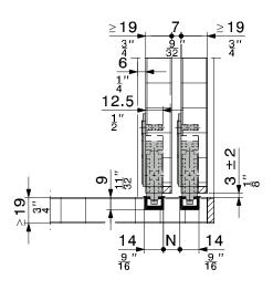
Hardware system for bottom running sliding cabinet doors with a weight up to 15 kg (33 lbs.) or 25 kg (55 lbs.).
