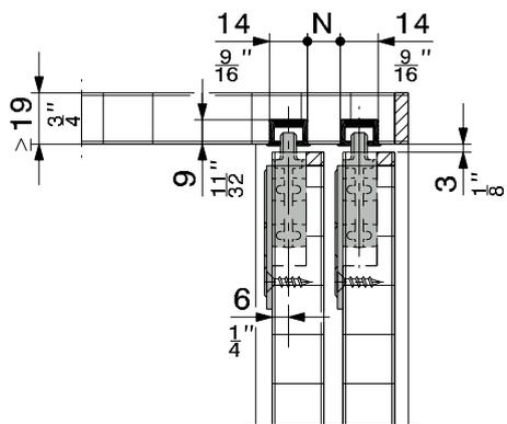
**Hardware system for bottom running sliding cabinet doors with a weight up to 15 kg (33 lbs.) or 25 kg (55 lbs.).**
