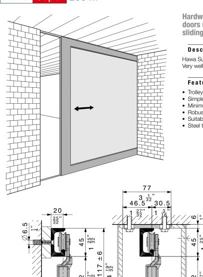
Hardware system for heavy weight metal sliding doors up to 250 kg (550 lbs.). Suitable for use with sliding fire doors.
