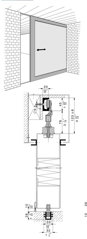
Hardware system for heavyweight metal sliding doors up to 500 kg (1100 lbs.). Suitable for use with sliding fire doors.
