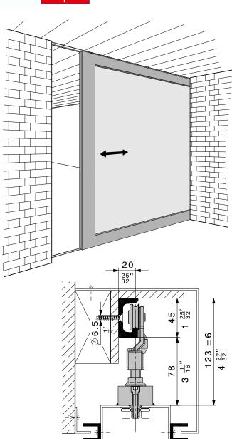
Hardware system for heavyweight metal sliding doors up to 500 kg (1100 lbs.). Suitable for use with sliding fire doors.
