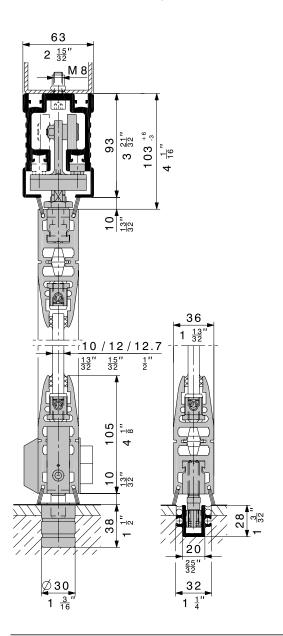
Frame profile for all-glass sliding walls up to 150 kg (330 lbs.) panel weight. Suitable for Hawa Variotec 150 GV.
